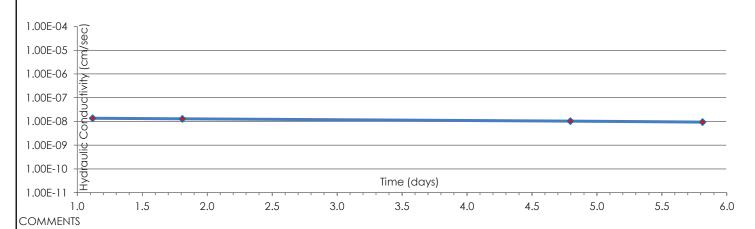
Shelby Tube recovered 59 cm of soil. Test sample portion taken from 30 cm to 40 cm from bottom end of tube.
